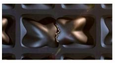
Take care while cleaning. If a substance has dried on the cushion and sticks cells together, do not attempt to separate the cells when they are dry. This may damage the cushion.
